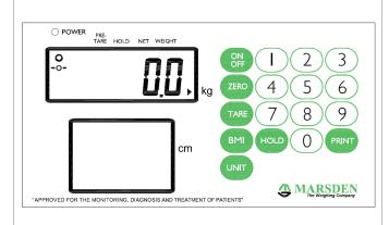
In normal mode, place a target that you want to tare off the weight (e.g. clothes) on the scale platform.
